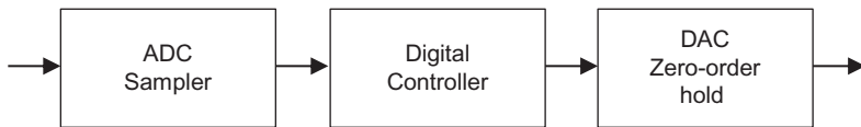
FIGURE 13.27 From ADC to the digital controller and then output to the DAC.
